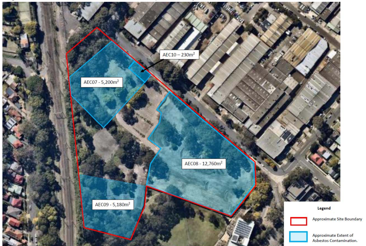
Figure 9: Areas impacted by asbestos contaminants.
